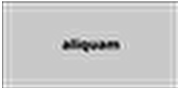
Figure 4: The original image was scaled down by a factor of 2 and then filtered by the sinc function with parameter T = 12 pixels.
